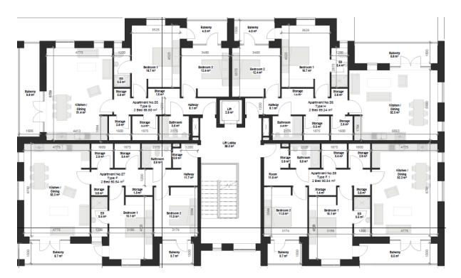
Figure 31.0 First and second floor plan for Apartment Block F. The ground floor plan of this block, which comprises the creche facility, is presented in Figure 81.0 of this report.
