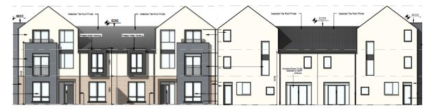
Figure 51.0 Front elevation of House Types 3.1-3.4 (left) and rear elevations of House Types 3.1-3.4 (right).
