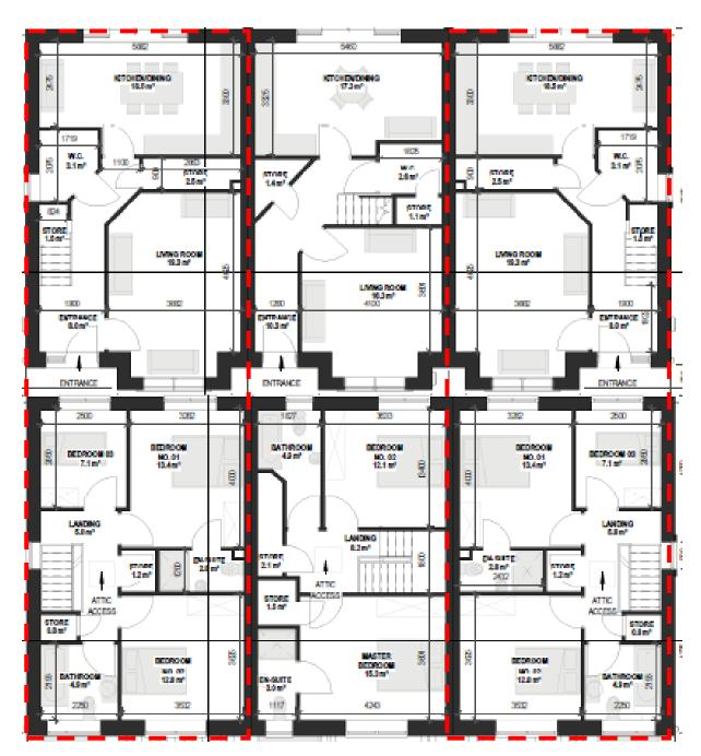
Figure 70.0 Typical ground floor plan of House Type 5.2 (top) and typical first floor plan of House Types 5.2 (bottom). The area within the red dashed lines represent the ground and first floor plans for House Types 5.1 & 5.3.
