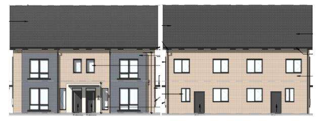
Figure 41.0 Front elevation (left) and rear elevation (right) of Maisonette buildings accommodating Maisonette Types 7.1-7.4.
