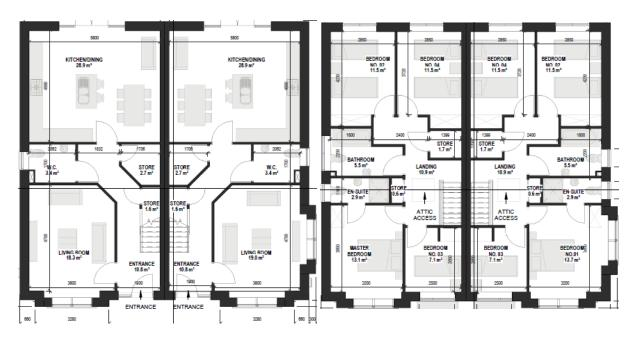
Figure 48.0 Typical ground floor plan of House Types 1.1-1.4 (left) and typical first floor plan House Types 1.1-1.4 (r).
