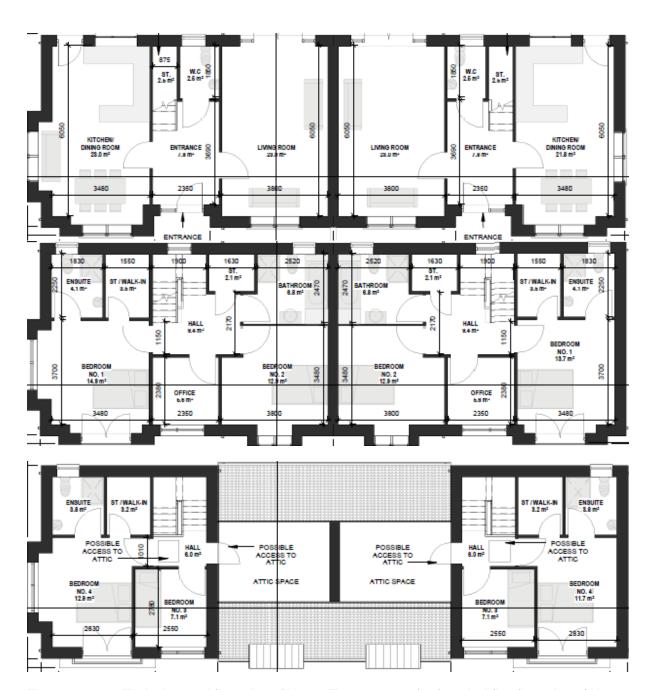
Figure 50.0 Typical ground floor plan of House Types 3.1-3.4 (top), typical first floor plan of House Types 3.1-3.4 (bottom) Types 3.1-3.4 (centre) and typical second floor plan of House Type 3.1-3.4 (bottom)
