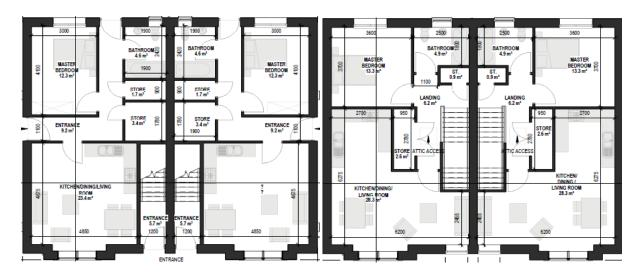
Figure 47.0 Ground floor level (left) and first floor level (right) of Maisonette buildings accommodating Maisonette Types 8.5-8.8.
