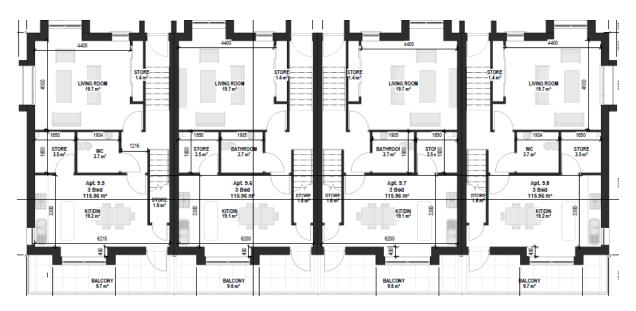
Figure 38.0 Second floor level of Apartments & Duplex Apartment Blocks, the first floor level of 4 no. duplex apartments is provided within each of the 2 no. blocks at this level.
