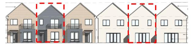
Figure 60.0 Front elevation of House Types 5.1 & 5.3 (left) and rear elevations of House Types 5.1 & 5.3 (right). The area within the red dashed line represents the ground and first floor plans for House Type 5.2.
