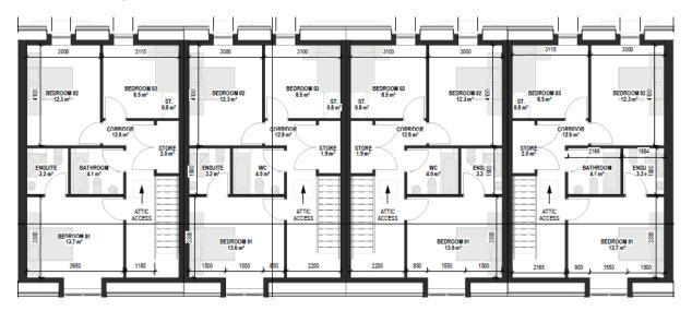
Figure 37.0 First floor level of Apartments & Duplex Apartment Blocks, the ground floor level of 4 no. duplex apartments is provided within each of the 2 no. blocks at this level.
