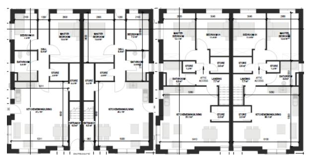
Figure 44.0 Ground floor level (left) and first floor level (right) of Maisonette buildings accommodating Maisonette Types 7.7-7.10.
