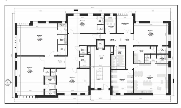
Figure 81.0 Proposed ground floor level of Block F illustrating layout of creche facility.
