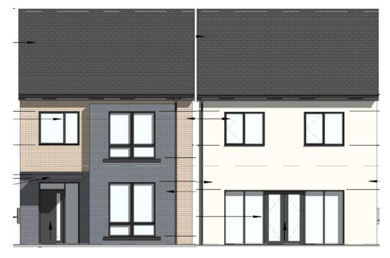
Figure 55.0 Front elevation of House Type 2.4(left) and rear elevations of House Type 2.4 (right).
