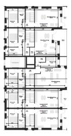
Figure 25.0 Second floor plan (left) of Apartment Block C and third floor plan (right) of Apartment Block C. As presented previously, only Building No. 2 of Apartment Block C rises above first floor level height.
