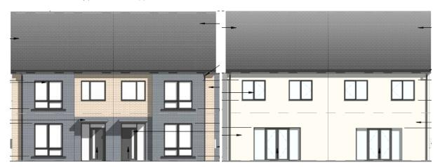
Figure 49.0 Front elevation of House Types 1.1-1.4 (left) and rear elevations of House Types 1.1-1.4 (right).
