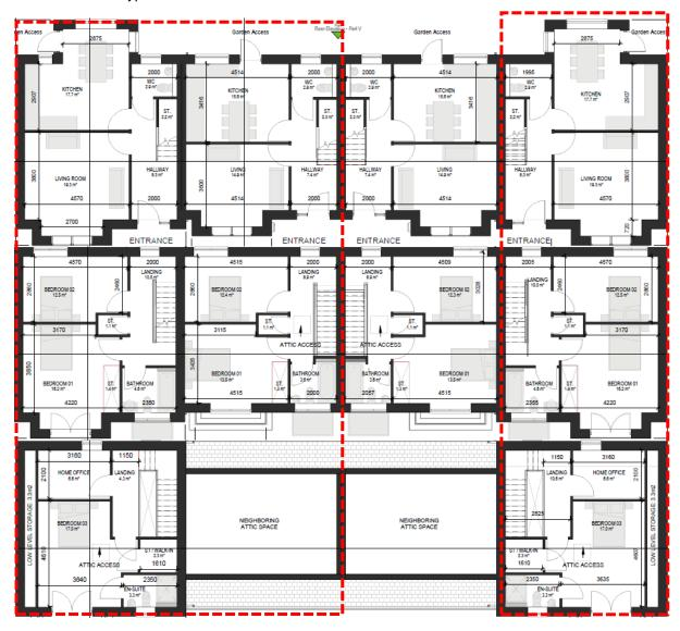
Figure 75.0 Typical ground floor plan of House Type 6.10 (top), typical first floor plan of House Type 6.10 (bottom). The area within the red dashed line represents the ground, first and second floor plans of House Types 6.1-6.3.
