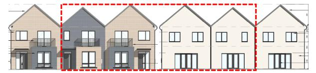
Figure 80.0 Front elevation of House Type 5.1 (left) and rear elevation of House Type 5.1 (right). The area within the red dashed lines represents the front and rear elevations of House Types 5.2 & 5.5.
